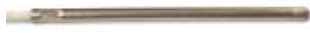
Part No. 3181-Lxx DIN A probe, steam-resistant, autoclavable, -200°C..180°C, LS = 100 mm, D = 5 mm
