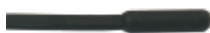
Part No. 3167-Lxx DIN B probe, -80°C..105°C, synthetic, molded, LS = 20 mm, D = 5 mm
